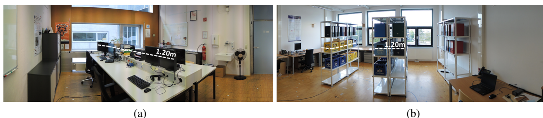
Figure 4.5: Evaluation setup (Image): Both rooms are filled with obstacles and scattering objects. The white dashed line marks the height under obstructed LOS. Adapted from [70].
